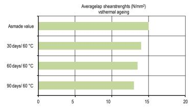
The tests have been carried out at 20  $^{\circ}\text{C}$  on steel to steel joints, which have been aged at 60  $^{\circ}\text{C}.$
