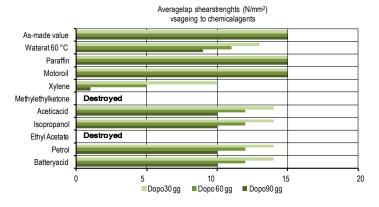
If not otherwise specified, the tests have been carried out at 20  $^{\circ}\text{C}$  after immersion for 30, 60 and 90 days at 20  $^{\circ}\text{C}$  on steel to steel joints which have been hardened for 48 hours at 20  $^{\circ}\text{C}$ .
