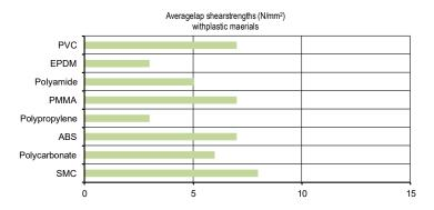
The tests have been conducted at  $20^{\circ}\text{C}$  on plastic to plastic joints, which have been hardened for 48 hours at  $20^{\circ}\text{C}$ .
