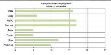
The tests have been conducted at  $20^{\circ}\text{C}$  on metal to metal joints, which have been hardened for 48 hours at  $20^{\circ}\text{C}$ .
